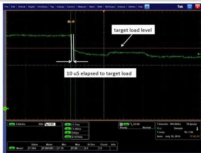
Figure 4.3.6: Rapid 10µs reaction to converter phase loss with cycle skip followed by DVFS.
